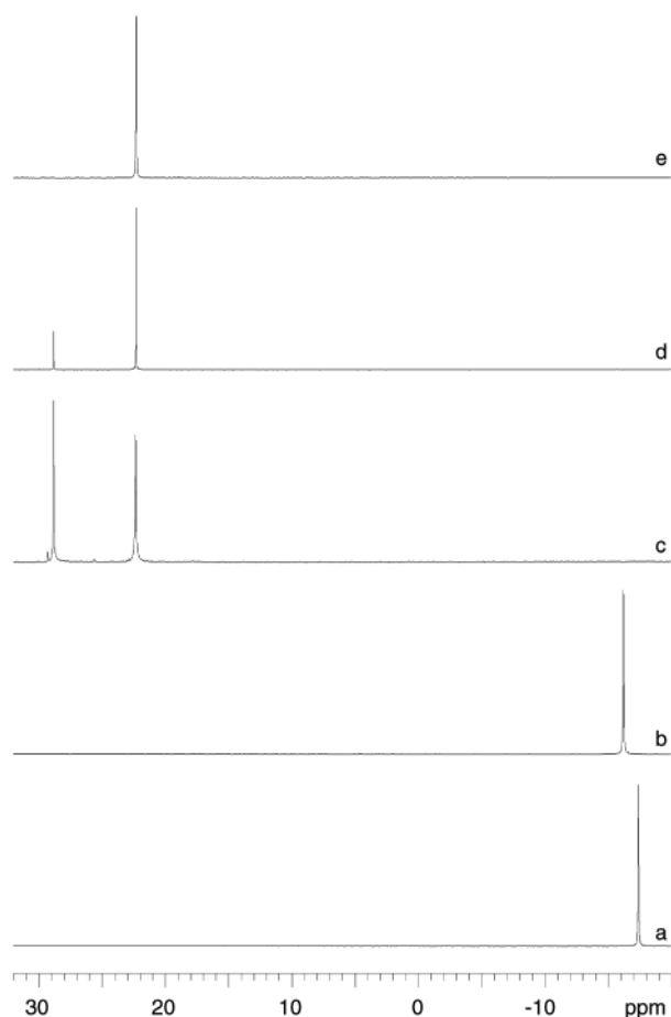
Fig. 3 ^{31}\text{P}\{^1\text{H}\} NMR spectra ( \text{CD}_2\text{Cl}_2 , 298 K) recorded to follow complex 5 formation: (a) (S_p) -Hpfc; (b) (S_p) -Kpfc prepared in situ from (S_p) -Hpfc and tert -BuOK; a mixture of (R_{Ru},S_p) - 5 ( \delta_P 22.3) and (S_{Ru},S_p) - 5 ( \delta_P 28.8) (c) after stirring (S_p) -Kpfc with [\{\text{RuCl}(\mu\text{-Cl})(\eta^6\text{-}p\text{-cymene})\}_2] for 3 and (d) after standing overnight; (e) spectrum of a recrystallized sample [several days, (R_{Ru},S_p) - 5 ].
